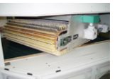
ROBA Tech brush belt for a perfect surface sanding in all areas
