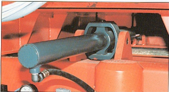
The hydraulic cylinder for the ram is mounted centrally in a
