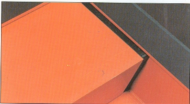
Synthetic gasket fills any void between Ram and hopper, thus avoids any material jamming.
