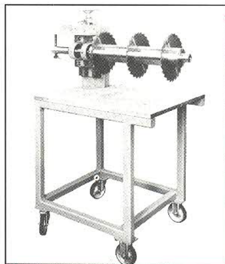
Transport cart with adjustable shaft for aid in removal of saw sleeve from machine and transporting sleeve to set-up area.
