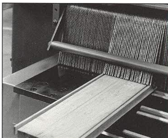
Close-up of ripped board leaving machine. First in the industry to provide outfeed anti-kickback fingers to prevent the edge trim strips from falling as they exit machine.
