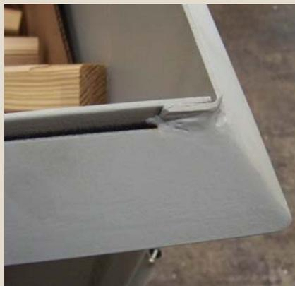
**Welded 2" reinforcing angle all along the top edge**
