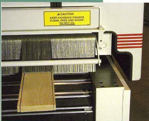
One additional row of outfeed upper anti-kickback fingers.
